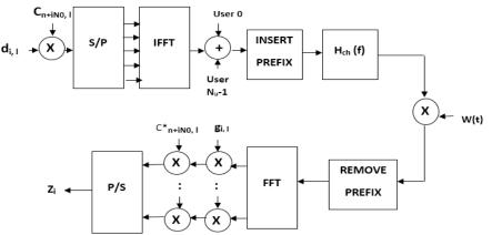
Figure 2: Block Diagram of Multi Carrier-Code Division Multiple Access system [7]
