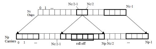
Figure 3: Mapping of chips on the carriers [7]
