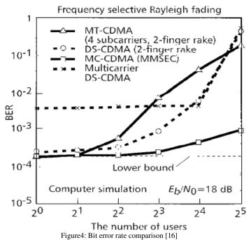
Compared to other multiple access schemes the main benefits of a MC-CDMA system includes high spectral efficiency, robustness to channel fading, flexible system design, high frequency diversity etc. However since MC-CDMA is a multi-carrier scheme, its performance is limited due to high PAPR, which occurs due to the combination of large number of independent subcarriers.
