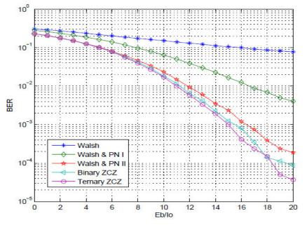
Figure 5: Bit error rate verses signal to noise ratio over Multipath Rayleigh fading channel [8]
